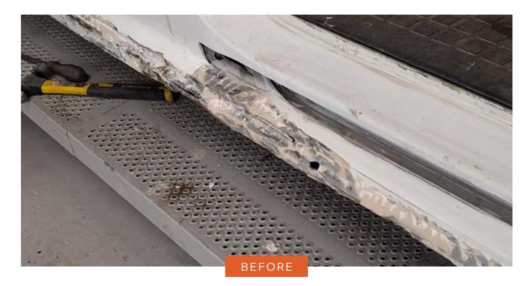
The N/S sill was poorly repaired, with filler covering extensive damage
