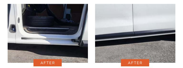
The damaged sill was carefully removed and replaced with new fabricated panels, restoring the vehicle at a much lower cost
